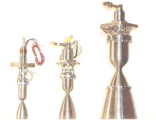
Fig.11 - A 22N, 50N, and 220 N HPGP thrusters From ECAPS's paper on "Expanding the ADN- based monopropellant thruster family"
