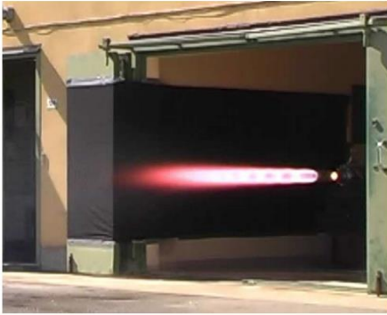
Fig. 6 - Test firing of ADN/GAP rocket motor. From FOI's paper on "Green Propellants Based on Ammonium Dinitramide (ADN)"
